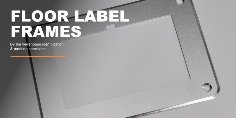
Floor label frames are made from CNC machined 1/8" and 1/16" aluminum sheet. Their design helps reduce impact damage with a beveled edge and rounded corners to reduce snagging. Screws are also counter sunk to prevent them catching on pallets, etc.
