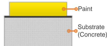
This is the solution chosen by more warehouse and distribution professionals than any other. It is produced with paint applied directly to a cleaned floor. Paint types may include acrylics, epoxies, and polyurethane's of varying performance capabilities and pricing.
