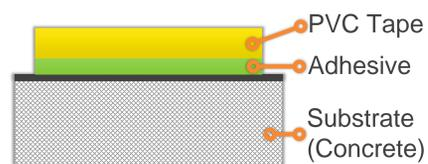
The method known by most people is a simple PVC tape applied to the floor for a quick, cheap and temporary solution.
