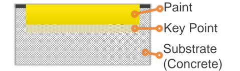
It's below the floor, FLT's and PPT's ride on to and off it, they cannot hit the side of the line, crack it or break the paint away.
